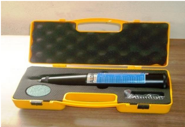
Figure 2.5 Rebound Hammer used for work
