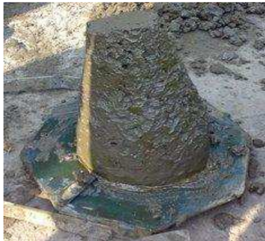
Figure 1: Fresh concrete after slump cone test
