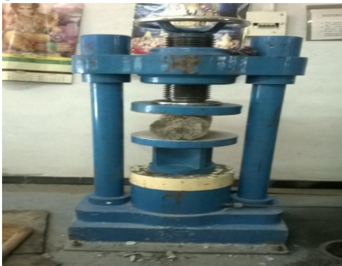
Figure 8: Split Tensile strength test
