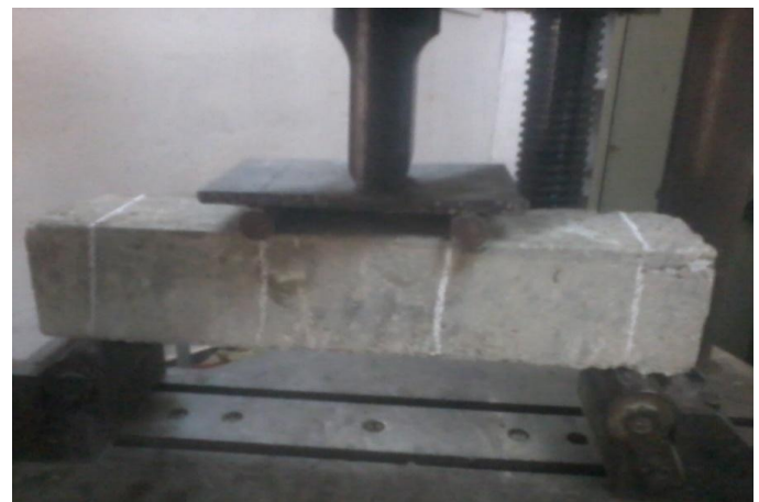
Figure 9: Flexural strength test
