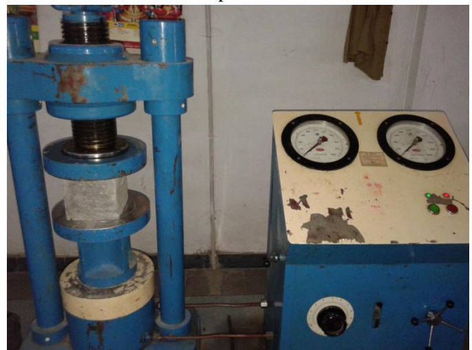
Figure 7: Compressive strength test
