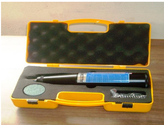
Figure:2.3(a) WTC-Model H Concrete Rebound Test Hammer is used in the present work.
