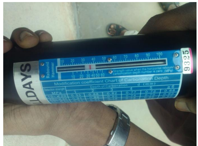
Figure:2.3(b) Taking reading of rebound value
