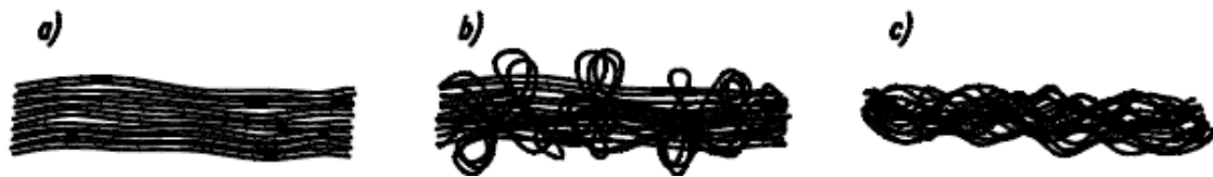
Fig.1. Various forms of roving: a) smooth roving, b) interlaced roving, c) tangle droving[5]
