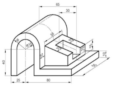
**OR 4.B. i)** Convert the following isometric view in to orthographic views. All dimensions are in 14M (BL2) millimeters.
