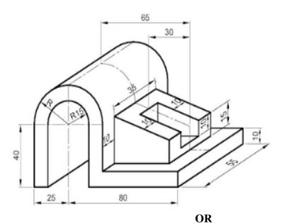
**4.B. i)** Convert the following isometric view in to orthographic views. All dimensions are in millimeters. **14M** (BL2)
