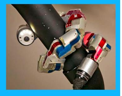
Snakes move rapidly through unstructured environments and avoid obstacles by going around or over them, or through small holes in the obstacle, such as a rock pile. For years, engineers have studied the remarkable locomotion capabilities of snakes to make snake-like robots that move in similar ways.
